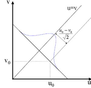
Figure 3. A 1D-Gaussian function is used to modulate the Sigmoid in the direction  $u=v$ . For a point  $(u_0, v_0)$  the Sigmoid function is modulated by the value of the Gaussian at the position  $(u_0 - v_0)/\sqrt{2}$ .
