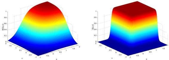
Figure 2. 2D-Sigmoid function for  $\beta_u=\beta_v=3$  and  $\beta_u=\beta_v=20$ .
