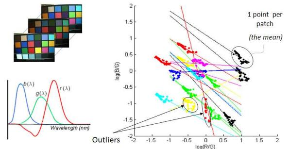
Fig. 4. Log-log space representation for all the patches of every acquired image. Every patch of each color in one image is represented using a single point, the mean. Cameras which do not use narrow-band sensors do not produce parallel lines for each patch.
