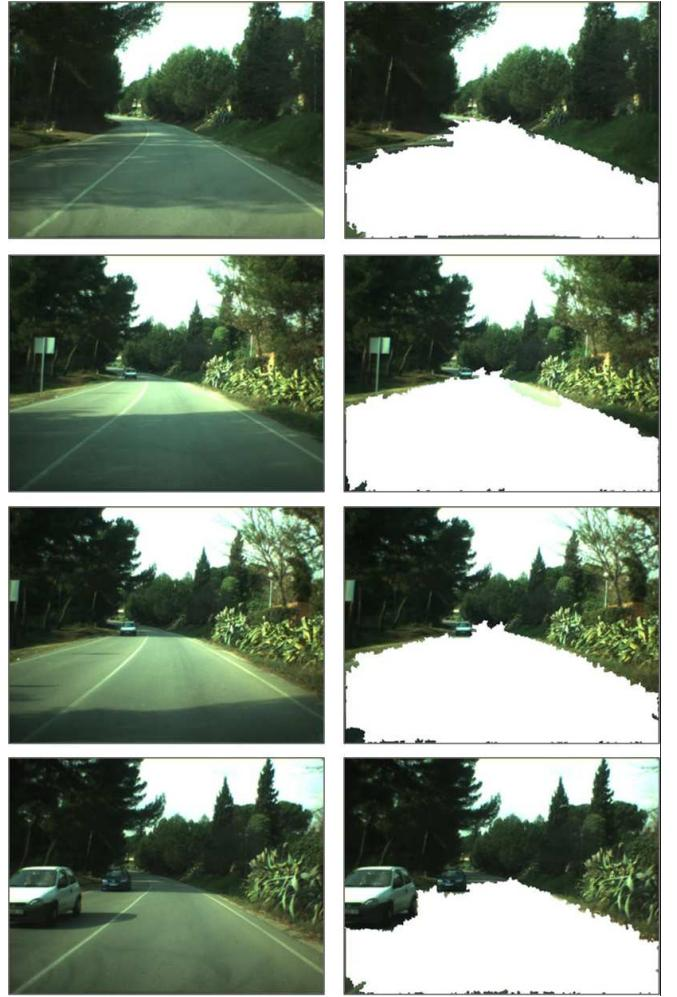
Fig. 12. Results from the sunny day sequence. This sequence includes extreme shadows and other vehicles in the scene. Left column is the original image which covers the nearest 80m ahead of the vehicle. Right column shows in white the corresponding segmented road.
