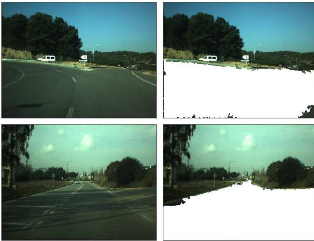
Fig. 14. Results with complex road shapes. Avoiding shape constraints allows the algorithm to segment the road surface even when the road is unstructured or with no clear shape.
