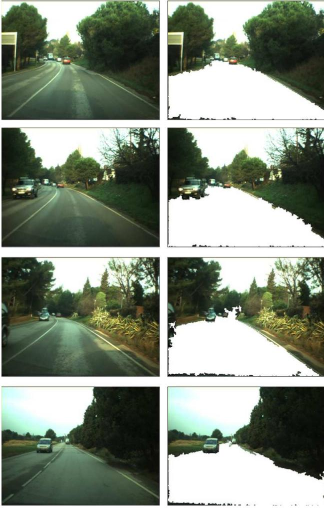
Fig. 13. Results from the rainy day sequence. Road surface is nonhomogeneous because it is non-uniformly soaked.
