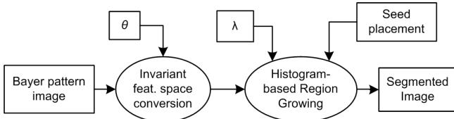
Fig. 11. Algorithm used to validate the road segmentation proposal.
