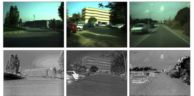
Fig. 3. Examples of illuminant invariant images. Upper row contains real images of different scenarios and the lower their corresponding invariant image. These results suggest the invariant theory holds although the theoretical assumptions are not perfectly achieved, i.e., the combination of our camera, the daylight illuminant and the surface we are interested in (the road).
