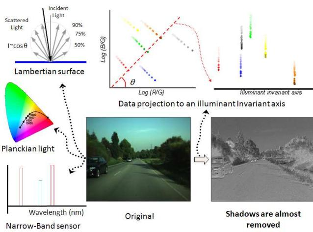
Fig. 2. Under the assumptions of Plankian light, Lambertian surface and narrow-band sensors, we can obtain an illuminant-invariant image which is almost shadow free.
