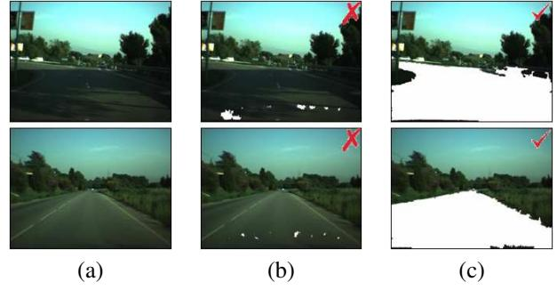
Fig. 8. Comparison of two different segmentations results when algorithms are applied to  $\mathcal{I}$  which is calculated from the original image as described in Sect. II. (a) Original image, (b) segmentation result using standard seeded region growing and the mean as dissimilarity criteria, (c) segmentation result using the histogram-based region growing algorithm.
