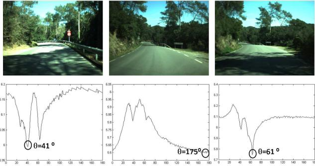
Fig. 5. Upper row shows some images used to calibrate the system by the entropy based method. Lower row shows their respective entropy distributions. These distributions vary considerably affecting the estimated invariant angle. These results suggest the method is not repetitive when used with real images.
