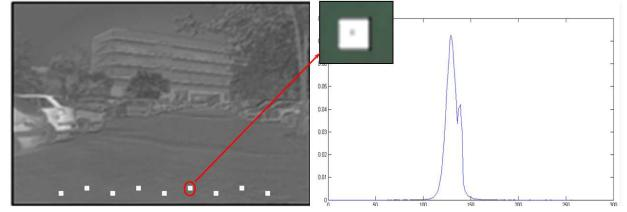
Fig. 7. Road model example: The model is built using the histogram formed with the surrounding region (white blocks) of several seeds. We have used nine seeds placed at the bottom part of  $\mathcal{I}$ .
