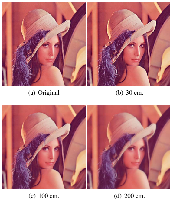
Figure 3. Perceptual color images of Lena performed by CIWaM. The lack of information does not produce compression artifacts, rather it is presented as a softened version.
